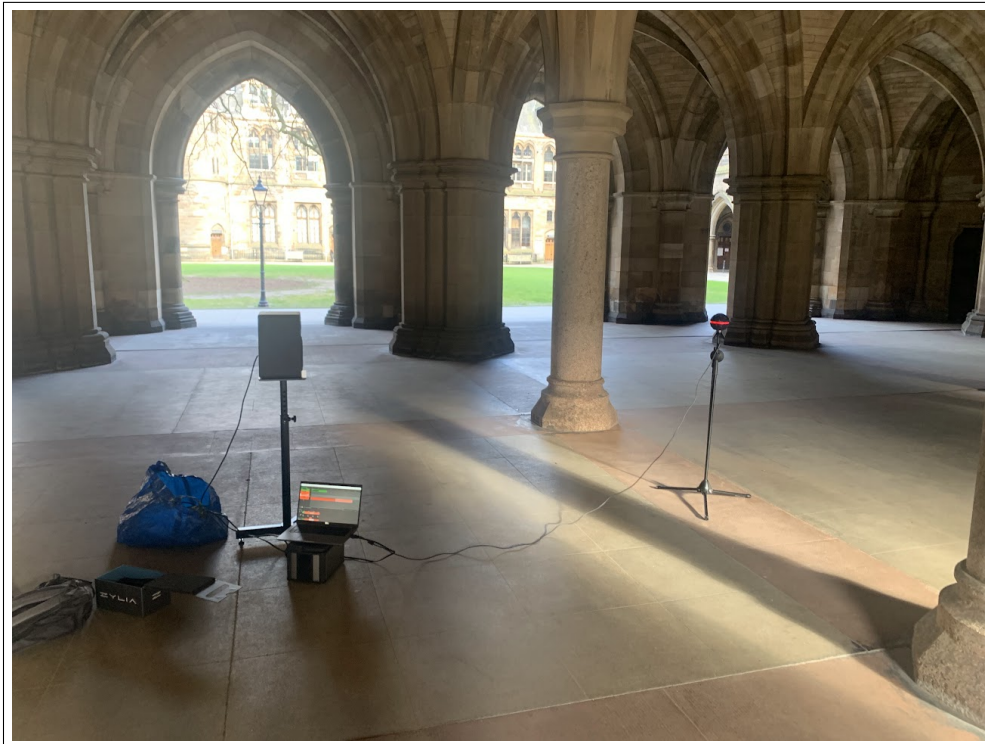
Figure 4.6: High reverberance test environment used for Study 2, illustrating the setup for RIR capture.
